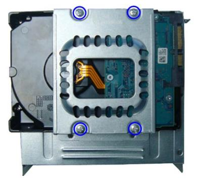
8. Slide the hard disk drive out of the bracket.
